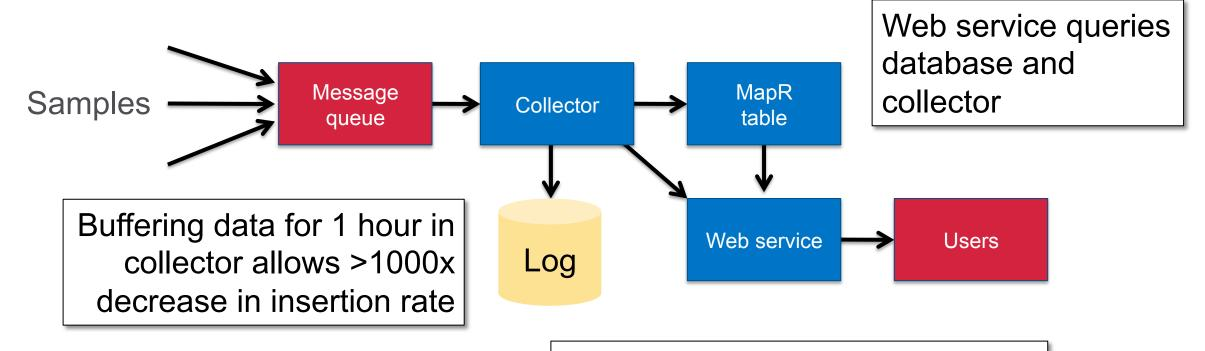
Logging latest hour of data allows clean restart of collector (lambda + epsilon architecture)
